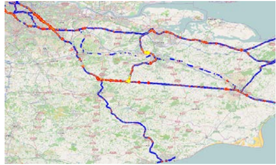
Figure: Condition map of the south east of the UK measured by Perpetuum equipped passenger trainsets
