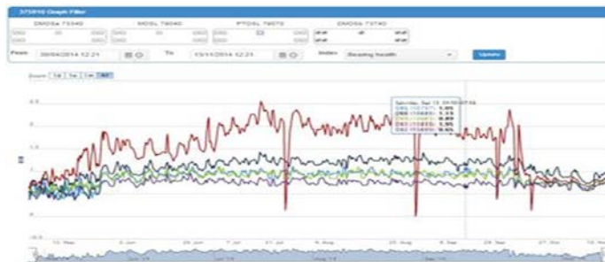
Figure: a wheel bearing being monitored over nearly 6 months of degradation prior to overhaul
